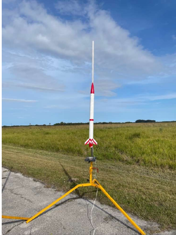
Figure 1 Fully integrated sub-scale rocket on the launch pad
