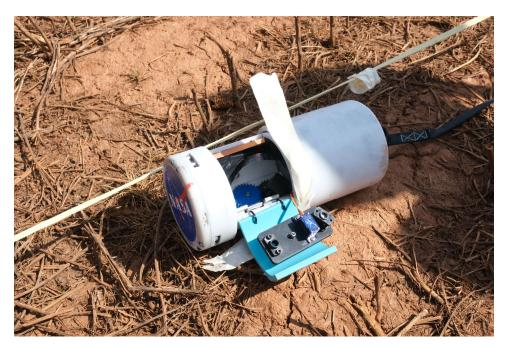
The core design of our payload proved to be fully functional in testing, able to orient itself, deploy the camera, receive radio commands, rotate 360-degrees, and record images. However, the PILL was only able to demonstrate some of these capabilities during launch.
