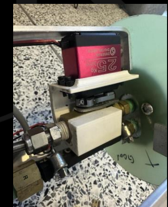
Mcmaster Compression fitting Brass check valve MOP 3000 & 2200 psi (1/4 & 1/2")
