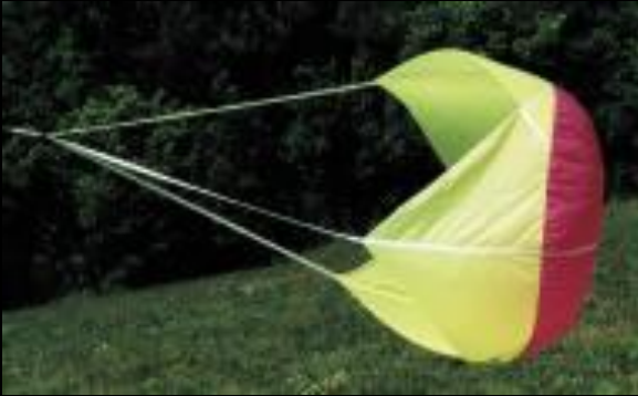
Drogue chute packing volume: Under 3 inches in length in a 6" airframe
