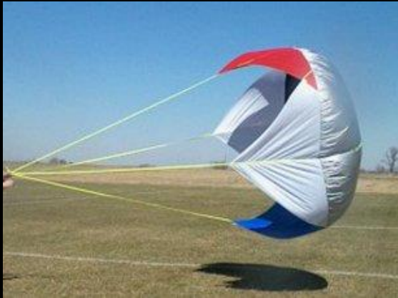
Drogue chute packing volume: Under 3 inches in length in a 6" airframe
