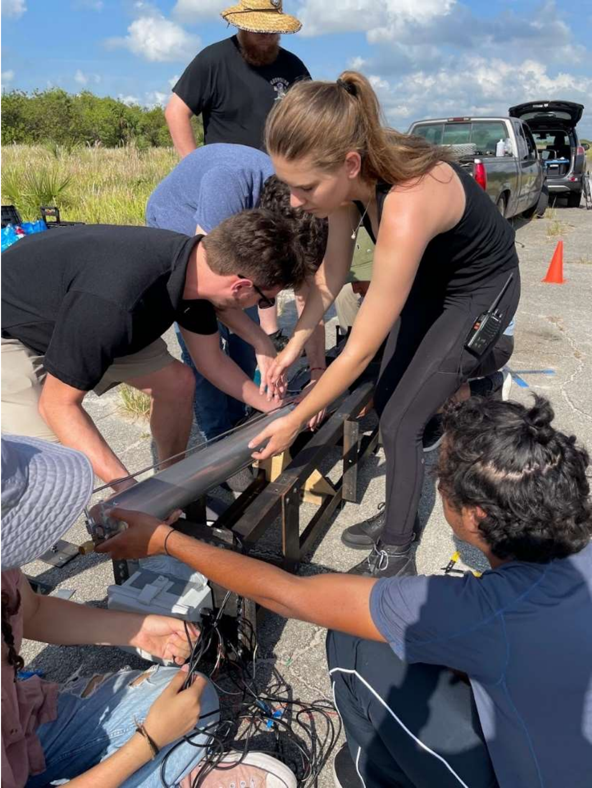
Photo of the Propulsion team securing the propulsion system for static fire testing.
